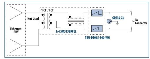
Gas tube devices are traditionally used as primary stage protectors in a multi-staged protection topology. In the circuit diagram shown above, the next-generation Model GDT35-23 gas tube is used in conjunction with a Model TBU-DT065-300-WH transient blocking unit high-speed protector (TBU® HSP) to protect a sensitive Ethernet PoE transceiver in an environment with exposure to induced lightning transients.
