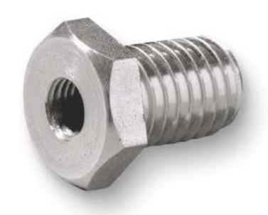
3M™ Disc Holder Adapter has both an interior threaded shaft and an exterior threaded shaft. The interior threads screw onto the shaft of a sander or other power tool, effectively increasing the size of the tool shaft, in order to accommodate a product with a larger center hole. It may be used with disc holders, discs, and other accessories with
