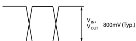
Figure 1a. Single-Ended Voltage Swing
