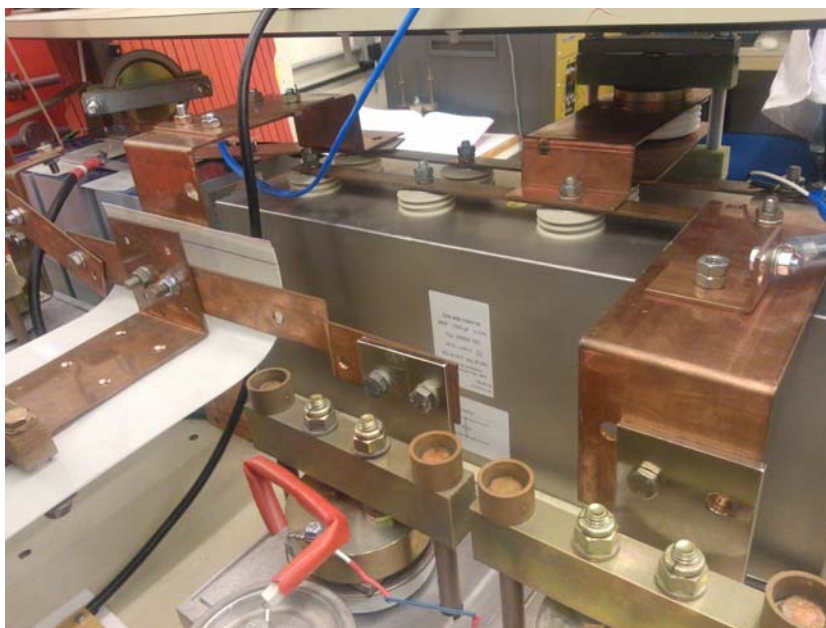
Capacitor E59.A66-10501W 1000 \mu F, 3kV DC Custom designed for use in IGBT switching circuit
