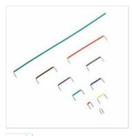
Wires are 22 AWG solid, tinned copper, PVC insulated, stripped 1/4 inch and bent 90 degrees on both ends for easy insertion.
