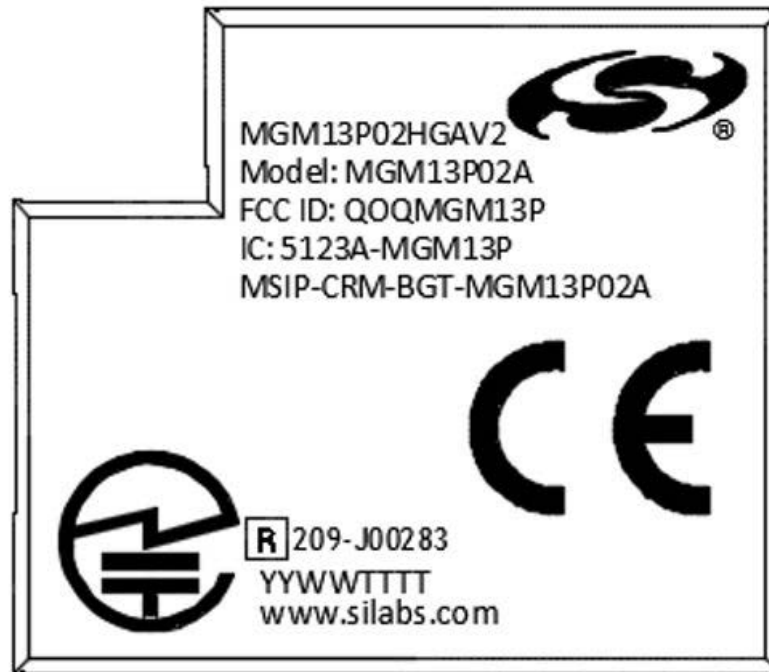
Figure 9.5. MGM13P Package Marking
