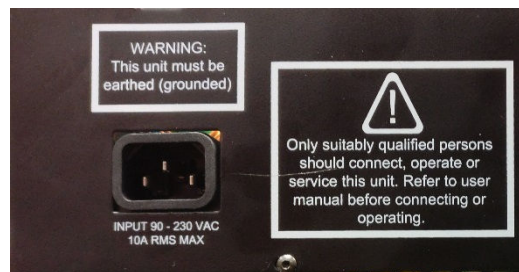
Figure 2-2. dsPICDEM MCHV-3 Development Board AC Mains Interface
