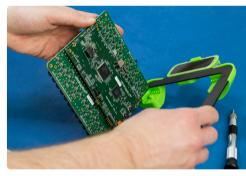
2. Separate the electronics board from the mounting frame
