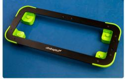
7. Unscrew all plastic parts from the square mounting frame. Using the 1.5mm Hex key, attach the corners to the rectangular frame. Leave the Leap Motion in its cradle and place aside for now.
