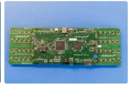
4. Position the control board onto the transducer array so that all four connectors are aligned.
