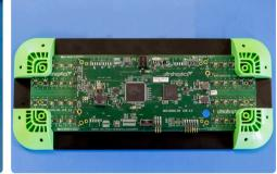
8. Position the board in the cradle with the power connector directed toward the Leap Motion cradle mounting holes.
