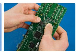
6. Apply pressure gently above each connector ensuring that the connections are secure.
