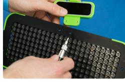
10. Using the 1.5mm Hex key, screw the Leap Motion cradle to the rectangular mounting frame.
