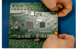
3. Position the UHDK5 with the transducers facing down on a flat surface. Place your fingers between the two boards and separate gently, working your way around until separated.
