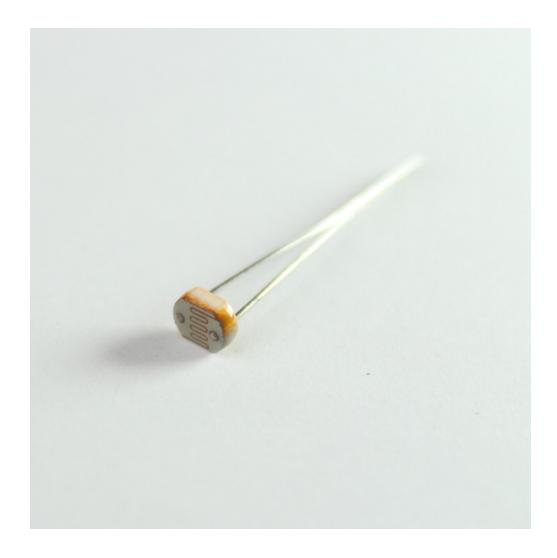
A photo resistor is a light dependent resistor whose resistance decreases with the increase in the intensity of light striking it. You can use it to detect the ambient light in the surrounding, detect shadows or use it as a part of a burglar alarm system. One photoresistor comes in your Photon Kit.
