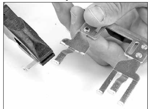
Figure 20: Prongs being broken off
