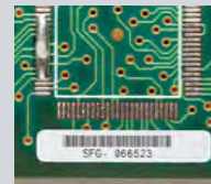
Circuit Board Identification
