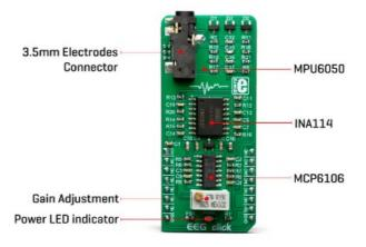
Since the "brain waves" can be both positive and negative, EEG click uses a virtual GND at the potential of 2.048V. This also helps reducing the noise from the common GND, improving the readings quality. The amplified brain activity signal is available at the AN pin of the mikroBUS<sup>TM</sup>, allowing sampling by the host MCU.
