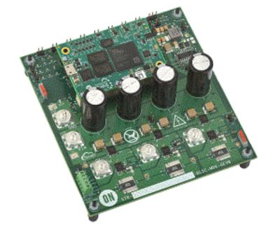
strategies and Al capabilities for industrial motor control. The complete kit is Strata enabled and the graphical user interface can be used to set control parameters for the motor drive.
