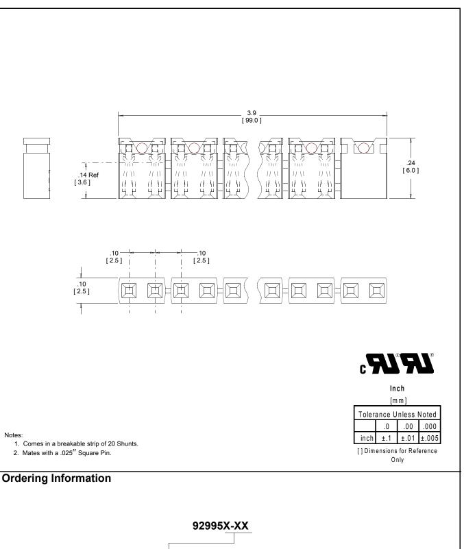
Color / Plating 1 - 00 RED / 75  $\mu$ " [ 1.90  $\mu$ m ] tin 2 - 10 BLUE / 75  $\mu$ " [ 1.90  $\mu$ m ] Nickel underplate, 10  $\mu$ " [ 0.25  $\mu$ m ] GOLD in the wipe area. 3 - 30 GRAY / 75  $\mu$ " [ 1.90  $\mu$ m ] Nickel underplate, 30  $\mu$ " [ 0.76  $\mu$ m ] GOLD in the wipe area.
