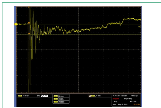
IEC 61000-4-2 -8 kV Contact ESD Clamping Voltage
